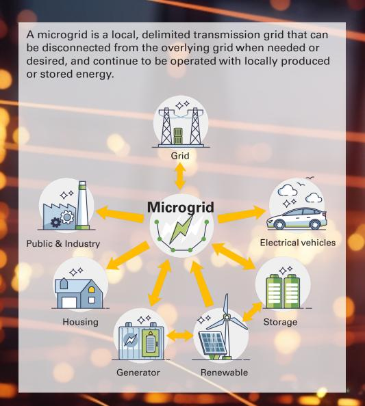
A microgrid is defined by three key characteristics:
