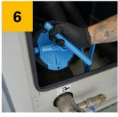
Remove the filter hatch by turning the hatch to the left and remove the filter.
